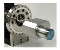
Consisting of XYZ table on CF150 for positioning sample holder and adjusting distance from target to substrate. Oxygen resistant heater is limited at a maximum temperature of 950°C. 0 to 60 rpm continuous rotation of the substrate. Manual or pneumatic integrated shutter following XYZ stage movements can be added.
