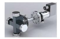
Consisting of XYZ stage on CF200 for positioning targets. Motorized Z-axis allows transfer on to the substrate manipulator. 0 to 60 rpm continuous rotation of the targets. Manual or motorized carrousel for sequential ablation.
